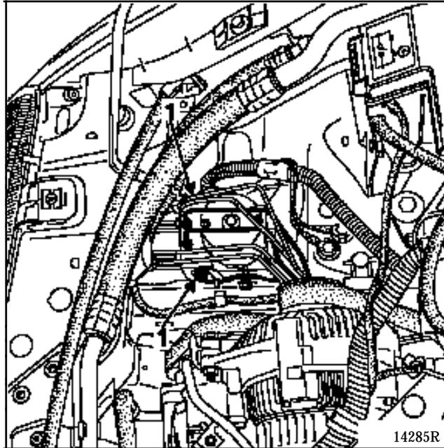
Remove the hydraulic assembly by slackening the two retaining nuts (1) (without removing them).
