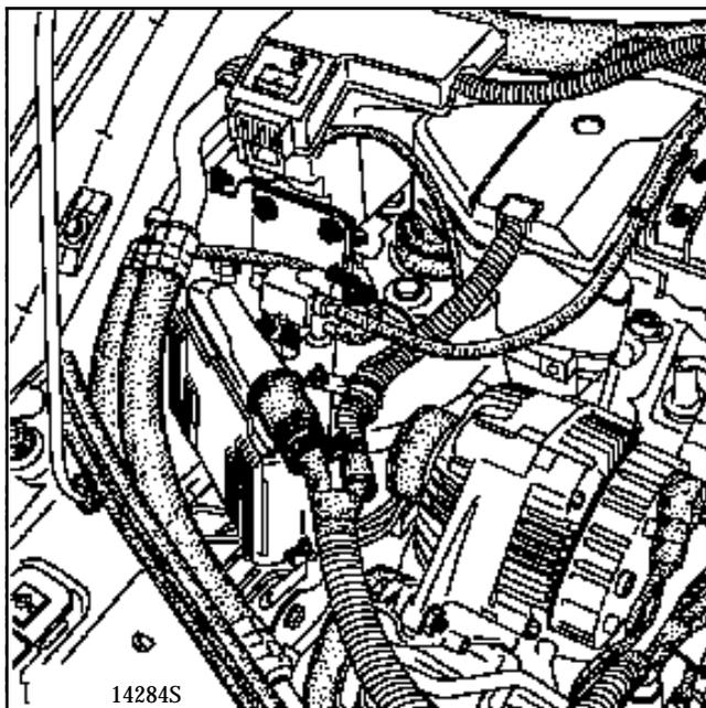
Lift the vehicle and disconnect the ABS computer connector by pulling the control collar.
