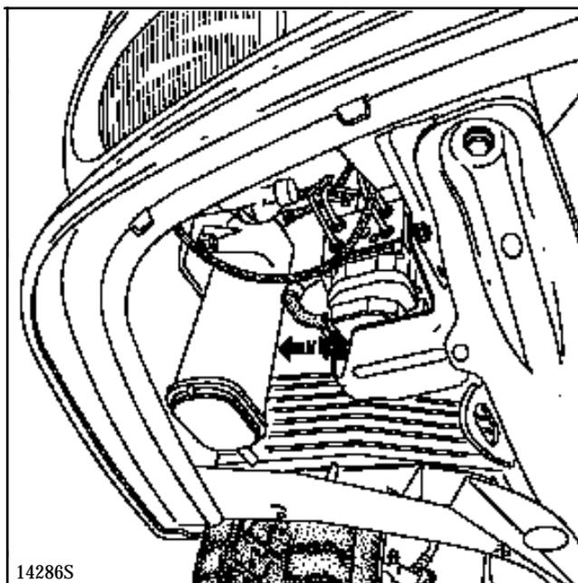
Disconnect the four hydraulic assembly pipes, mark their position for refitting.
