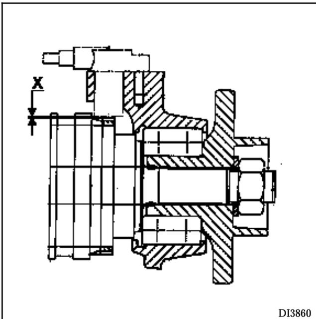
The air gap can only be checked on vehicles equipped with rear disc brakes.
