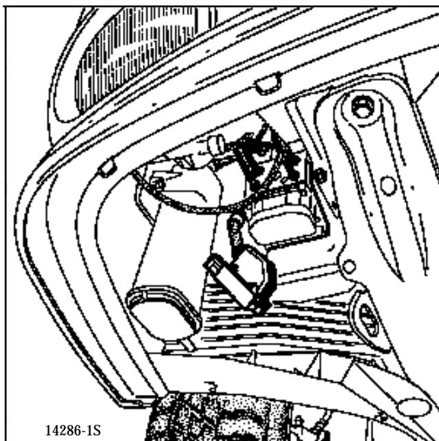
Lower the vehicle and disconnect the two hydraulic assembly pipes.
