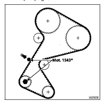
\* Mot. 1543-02 with intermediate shaft Mot. 1543-03 without intermediate shaft
