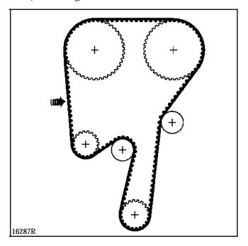
Point for pretensioning and/or checking belt tension
