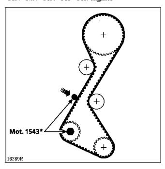
\* Mot. 1543-02 with intermediate shaft Mot. 1543-03 without intermediate shaft
